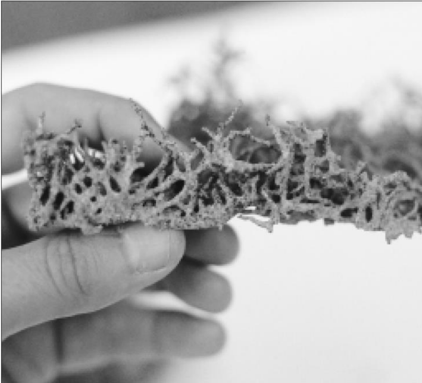
ABOVE: Timber devastated by a termite attack (As shown above)
