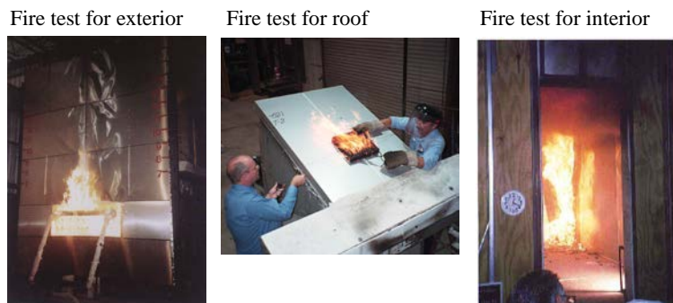
Fig. 1-6 Examples of fire tests applied to ALPOLIC/fr
